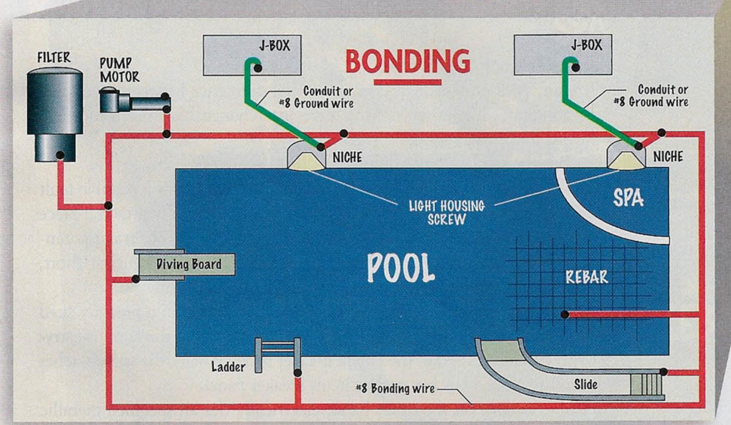
Red bonds together: Bonding minimizes the differences in potential, or voltage, between metallic components around the pool to reduce shock hazards. Anything metallic within 5 feet of the inside pool wall (including the rebar and conductive deck materials) should be tied to the bonding grid. (Note: The wires running from the light niche and terminating at the junction box are technically grounds and therefore green. However, they also serve as bond wires.)
